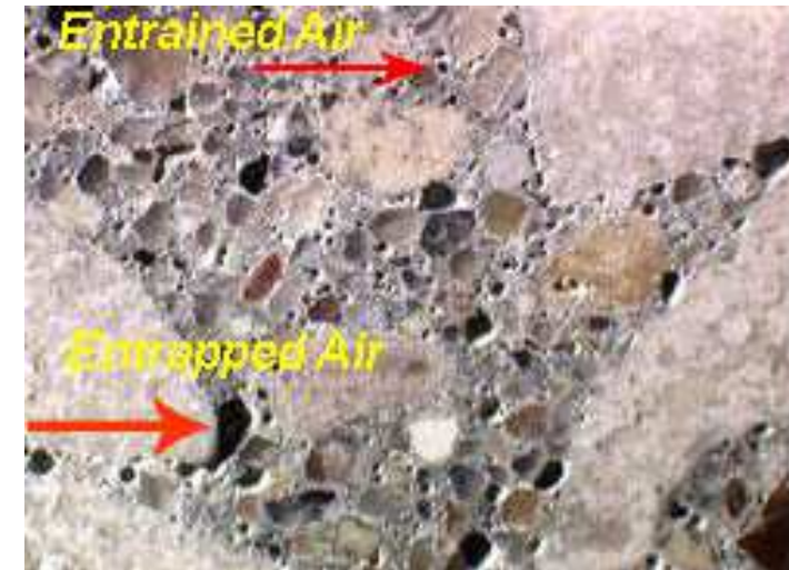
Optical microscope image of an air entrained concrete
